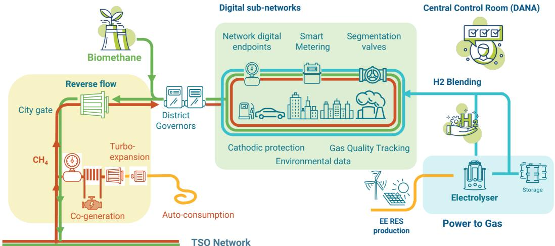
in the next years. The repurposing of the network sees, among other things, the full replacement of pipelines, risers and plants made of grey cast iron, unprotected steel without cathodic protection system and other obsolete materials, guided by predictive maintenance principles, avoiding gas leakages in atmosphere and allowing green gases injection in our network. To deepen our smart maintenance project, please see Par. 2.3.
